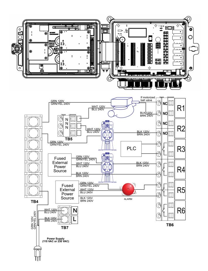
Figure 15 W610 AC Power & Relay Output Wiring
