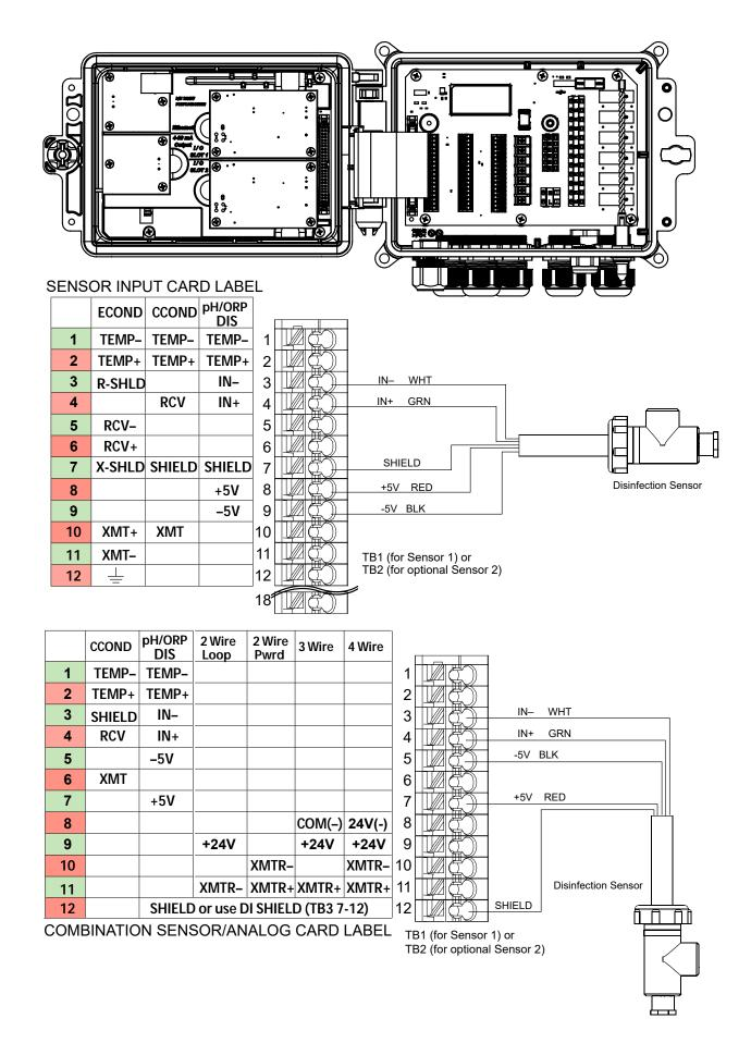
**Figure 10 Disinfection Sensor Input Wiring**
