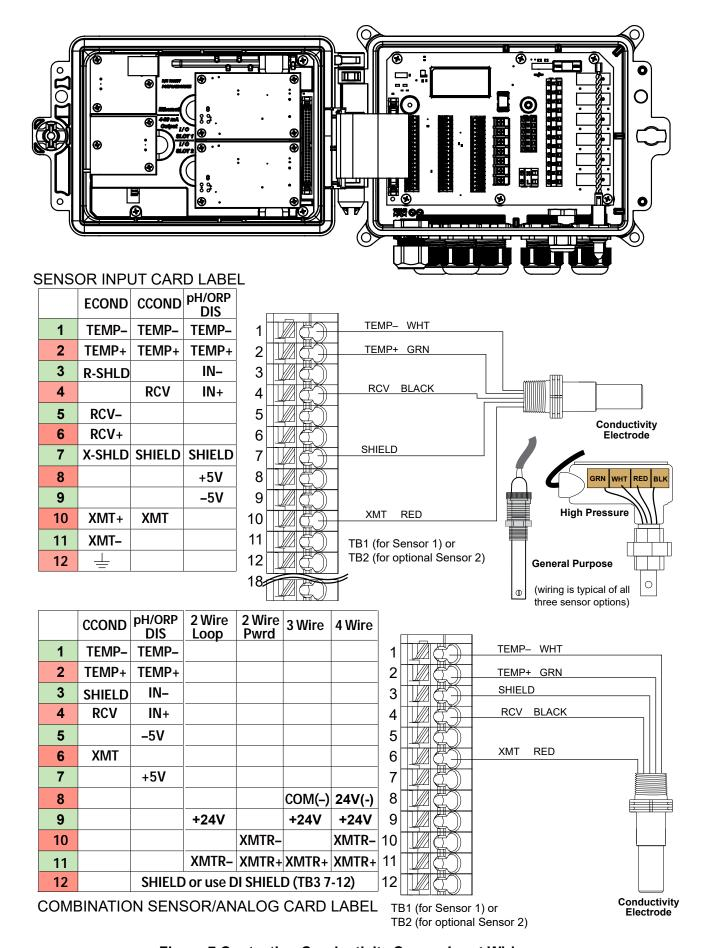
Figure 7 Contacting Conductivity Sensor Input Wiring
