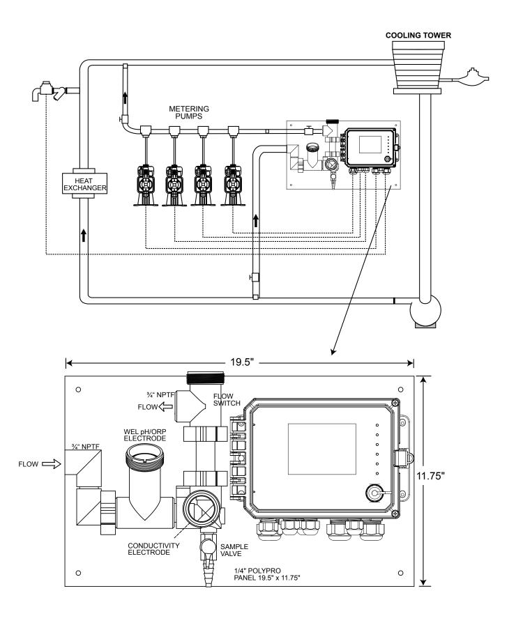
Figure 1 Typical Installation – Cooling Tower
