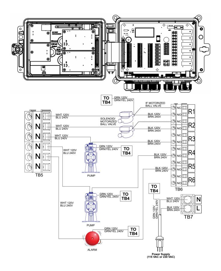
Figure 14 W600 AC Power & Relay Output Wiring
