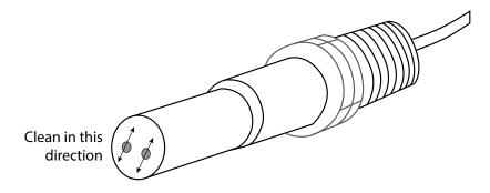
Figure 20 Cleaning the Electrode
