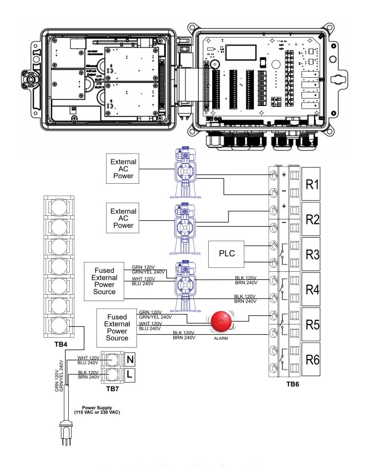
Figure 16 W620 AC Power & Relay Output Wiring
