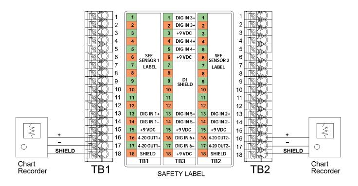
**Figure 18 Analog Output Wiring**
