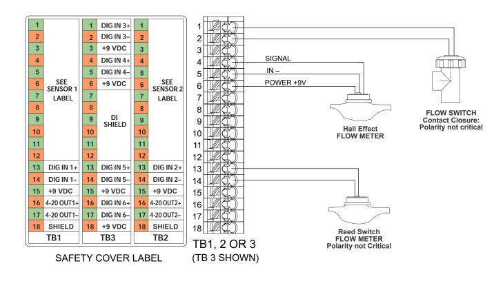
**Figure 13 Digital Input Wiring**
