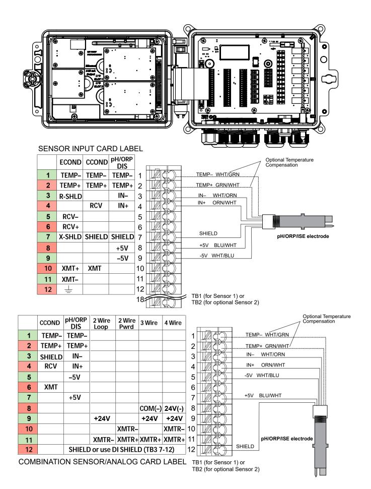
Figure 9 pH/ORP/ISE Sensor Input Wiring
