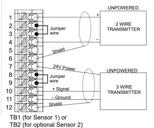
Figure 11 Dual 4-20mA Sensor Input Wiring
