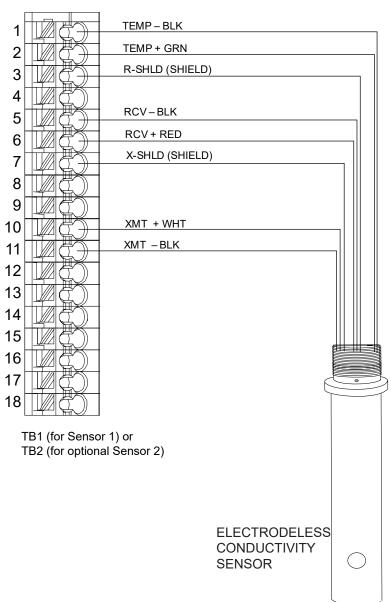
Figure 8 Electrodeless Conductivity Sensor Input Wiring
