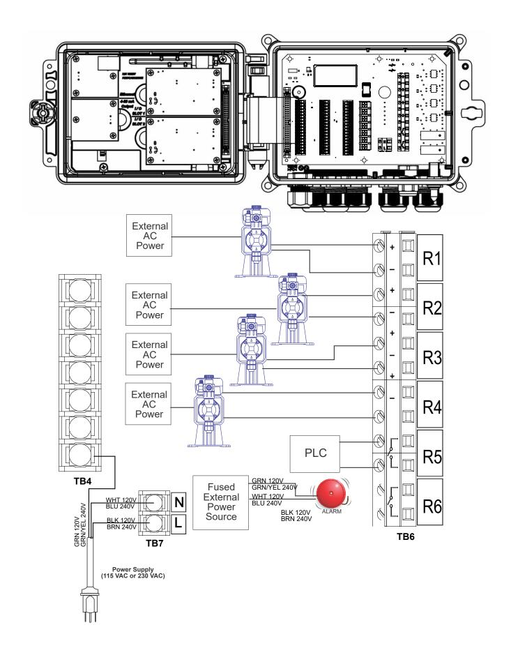
Figure 17 W640 AC Power & Relay Output Wiring
