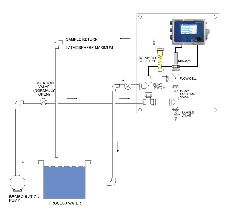
Figure 3 Typical Installation – Disinfection Sensor
