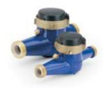
water. The WFM Series uses the widely recognized multi-jet principle, which has been accepted as an international standard for many years. These meters are available with either a two-wire reed switch, or a solid state, three-wire Hall effect sensor.
