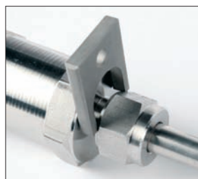
Properly tightened, the gauge will not fit
