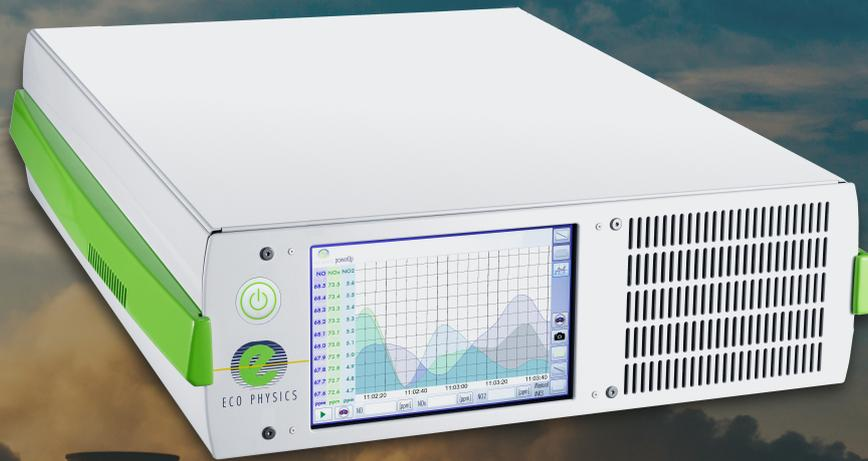
**The nCLD 822 CMh analyzer is the next generation in high precision nitrogen oxide measurement. Unique in speed and reliability, the nCLD 822 CMh is modular designed and capable of sequentially measuring NO, NO<sub>2</sub>, NO<sub>x</sub>, NH<sub>3</sub> and NO<sub>x</sub>-Amines from hot and humid gas sources without additional cooler. The new and intuitive graphical user interface also individually displays and connects to other instruments' data.**
